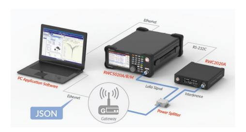
Fig 3.30 Interferer test environment
