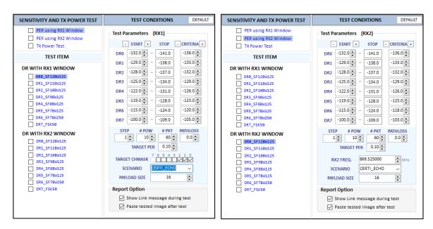
Fig 3.11 Test Conditions for PER using RX1 and RX2 Window
