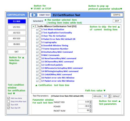
Fig 3.1 Test function window for LoRaWAN pre-certification.
