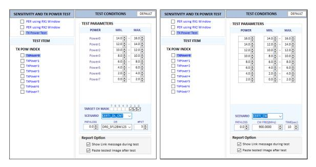
Fig 3.12 Test Conditions for TX Power Test using Lora signal or CW
